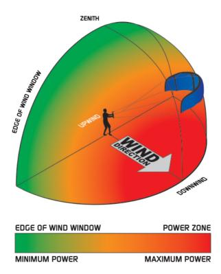
Before flying your kite it is very important to understand the 'wind window'. The image shows where the kite will create the most power (straight downwind, also known as the 'power zone') and where the kite will create the least power (edge of the window and zenith).
